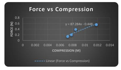
The slope of the line is the value of spring constant (k in N/m). This is calculated using the following formula.
